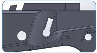
ENSURE THAT THE DRILLED CHANNELS ARE TOTALLY CLEAR OF ANY REMOVED MATERIAL BEFORE INSTALLATION OF PARTS KIT
