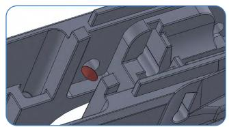
REMOVE ALL BURRS FROM THE INSIDE SURFACES NEAR THE DRILLED HOLES BEFORE INSTALLATION OF PARTS KITS
